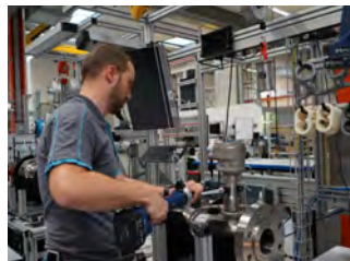
Also designed with ergonomics in mind: the new assembly workplace based on the VDI 2862-2 directive.
