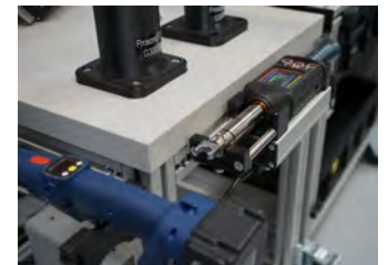
Immediately accessible: offset drivers from HS-Technik and torque/offset wrenches from SCS Concept.
