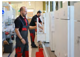
After fully automatic parts production, the front panels, drawers and equipment are assembled manually.
