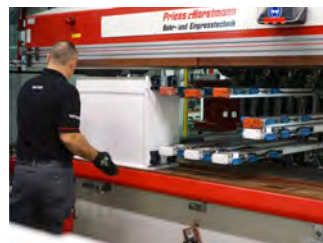
Assembly highlight: This furniture press assembles a cabinet every 30 seconds.
