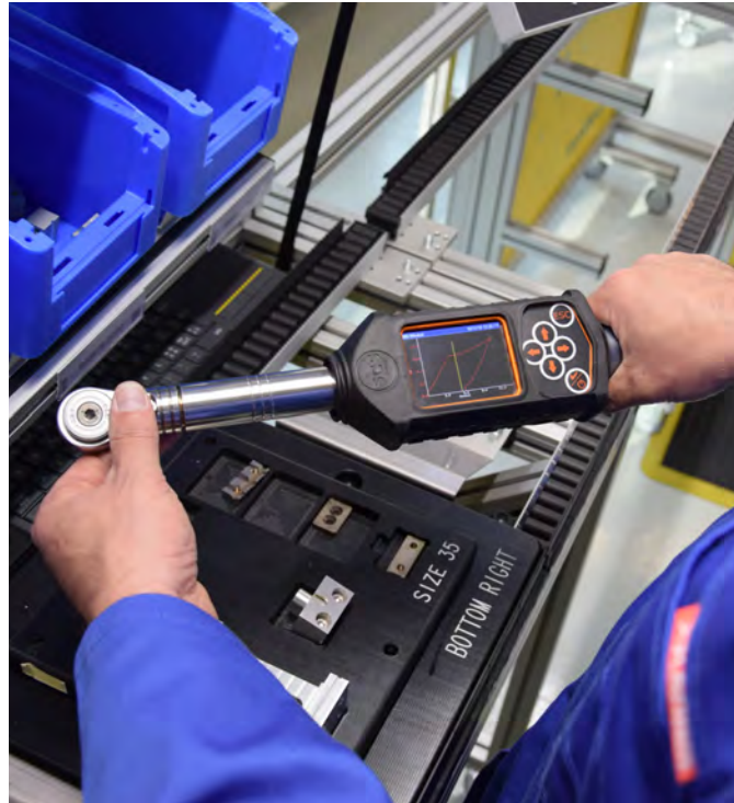
Process capability test on the assembly line.
