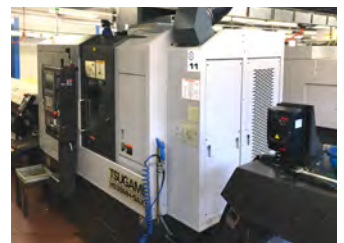
This Tsugami system manufactures extremely complex parts on five simultaneous axes.
