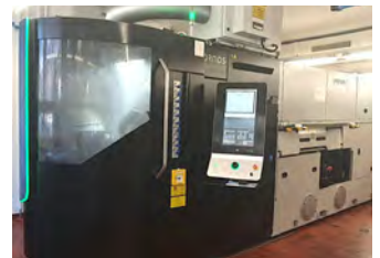
Five times as fast as a single spindle: this multi-spindle machine performs six processes simultaneously.
