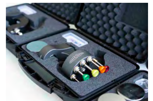
Renowned for high precision: A rack press specially developed and produced for the watchmaking industry.
