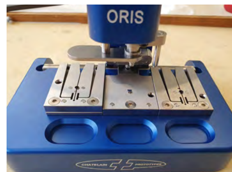
For reliable fine adjustment during assembly: Tool for a watch regulator system.
