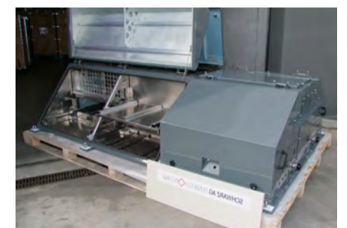
Aluminium converter housing for a locomotive roof: Contains the drive and control electronics.
