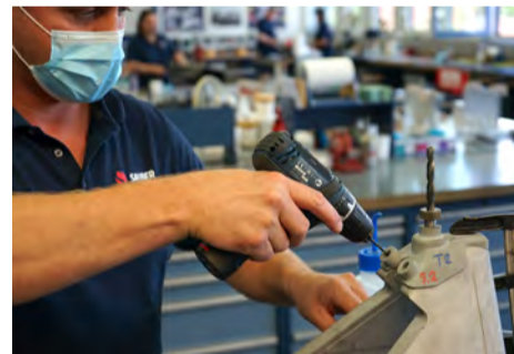
Equipped by Brütsch/Rüegger Tools: Drilling process on the roll cage made of 3D-printed aluminium.
