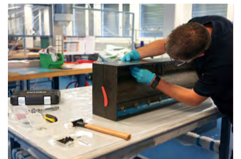
For fine surfaces: Both forms are compressed and excess resin is squeezed out.
