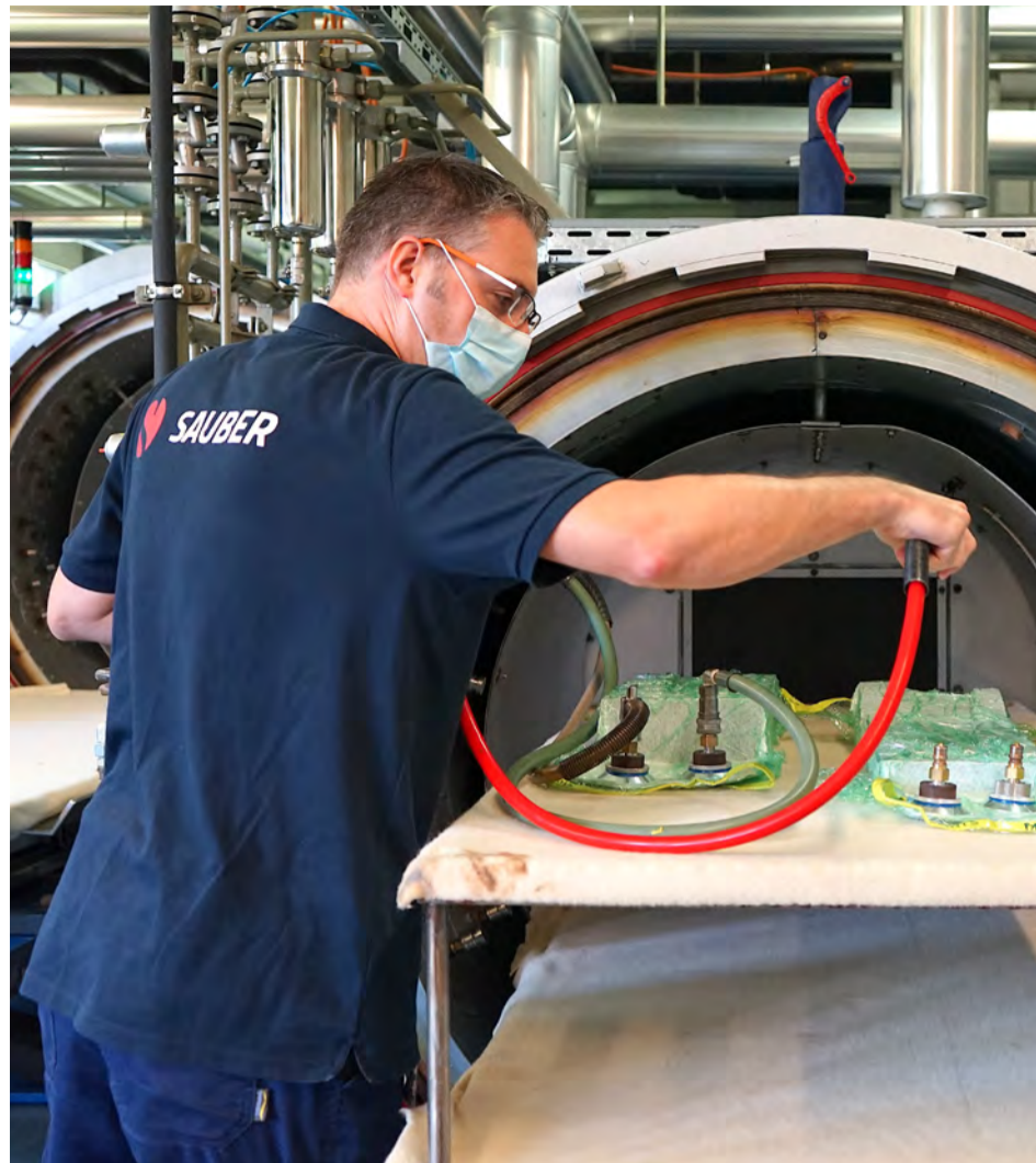
The highest process reliability: Before curing in the autoclave, the carbon parts are again carefully vacuumed.
