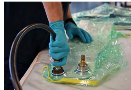
Before curing, CFRP components are packed in non-woven fabric and vented in a vacuum bag.
