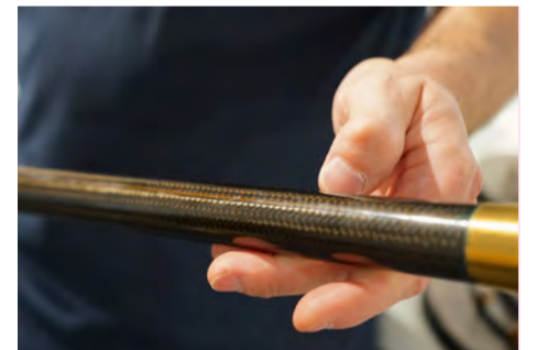
A true lightweight: A carbon fibre steering column made by Sauber Motorsport.
