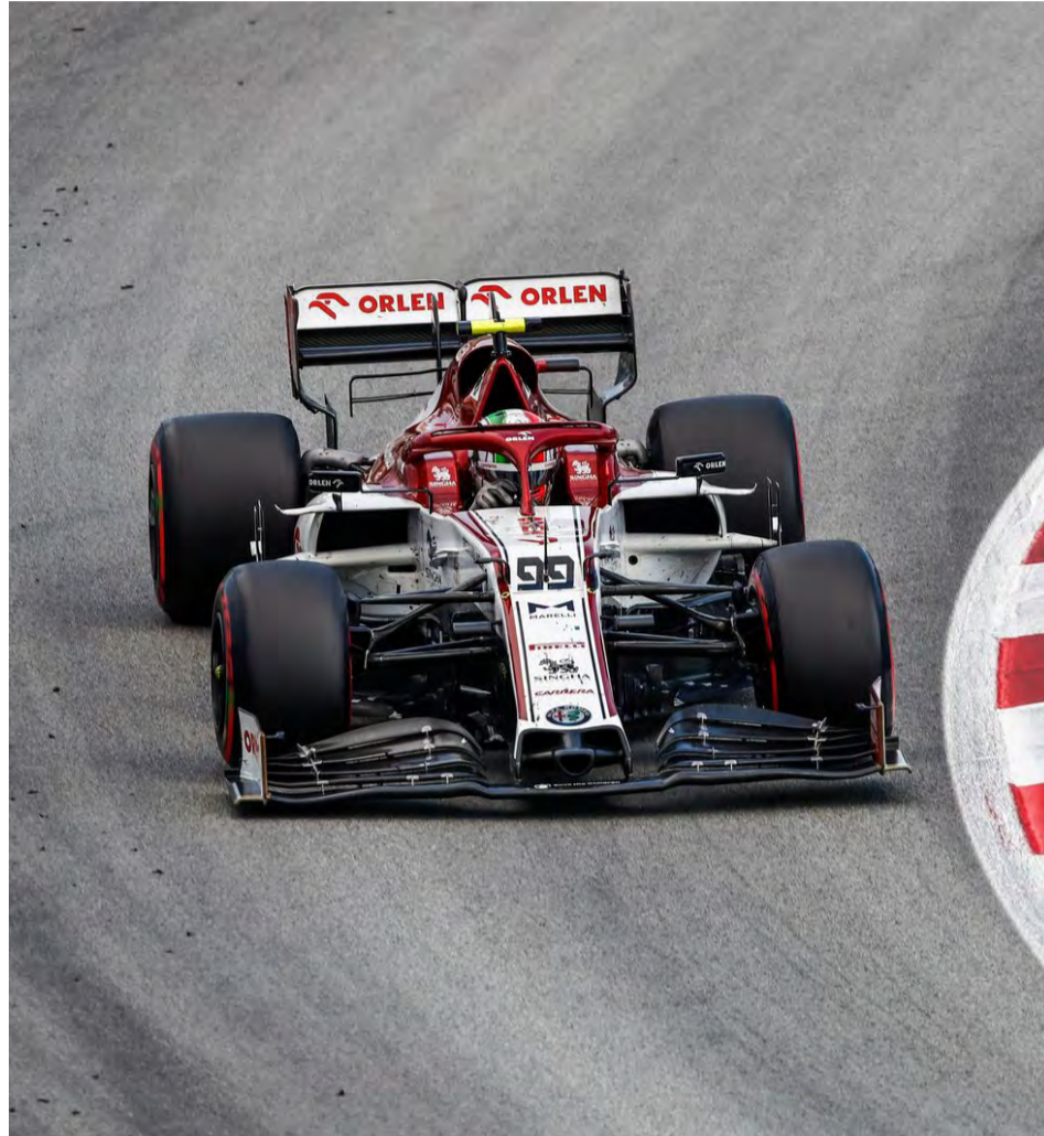
Hybrid drive: The C39 has a 1.6-litre V6 (Ferrari) turbocharged engine and a 120 kW electric motor.
