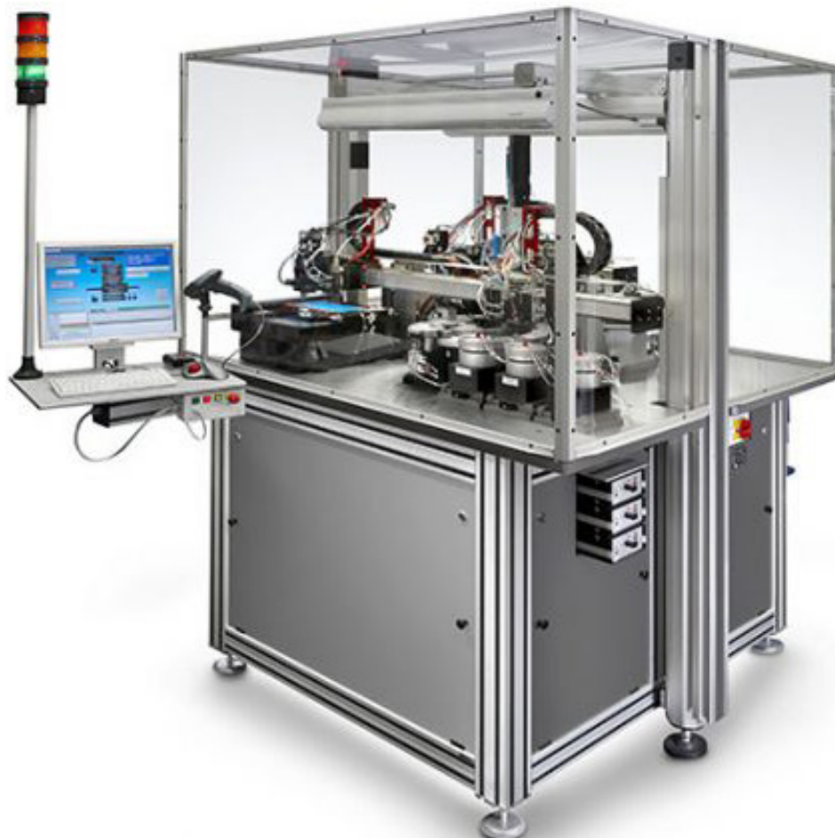
Automated assembly system for easier assembly of watches and movements.
